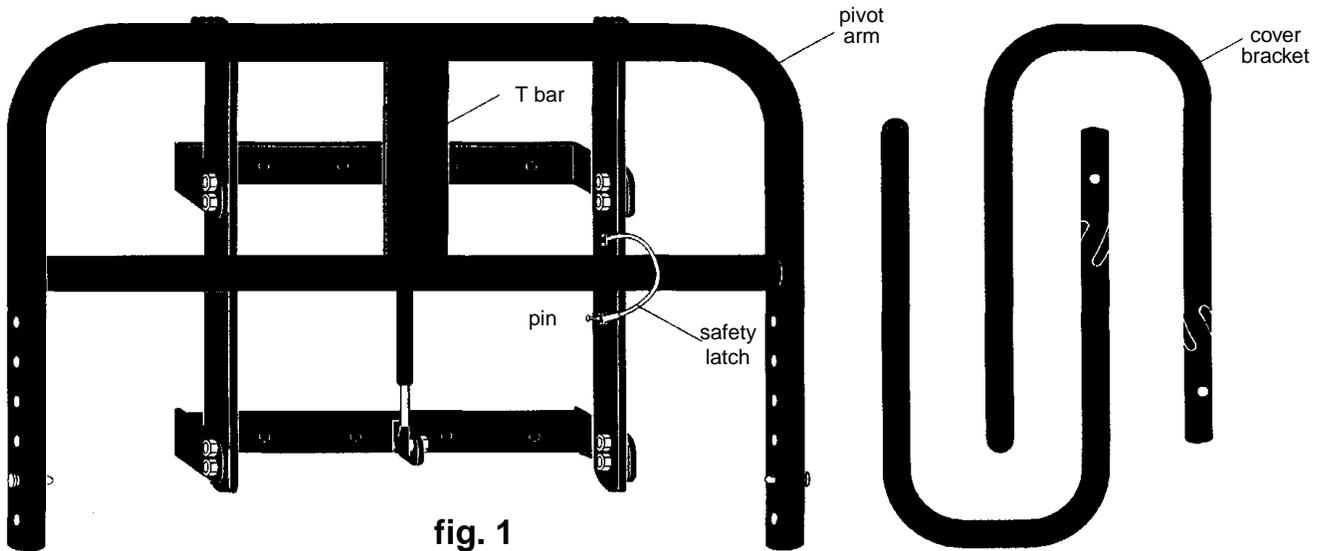
2. Position Cover Caddy centered side to side on spa cabinet (on side of spa with 3' clearance). Pivot arm must be even with top rim of spa. Use the 8 wood screws provided when mounting Cover Caddy through the 8 holes on the 2 support bars. **MAKE SURE YOU ARE MOUNTING TO SUPPORT BEAMS (under outside cabinet).** IF you cannot locate support beams or none are available to mount to, mount (2) 2x2 wood sticks to spa cabinet first, then mount Cover Caddy to 2x2s (fig.3).
